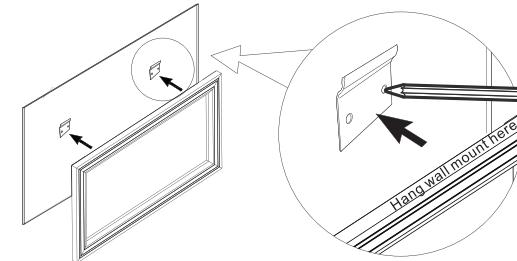
Fix the wall mount at the place where stickers on frame point out.
