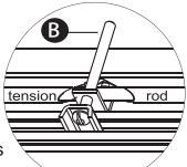
Tighten the tightening screws to make the screen flat.
