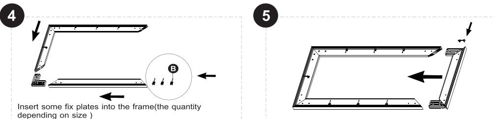
Insert some fix plates into the frame(the quantity depending on size )
