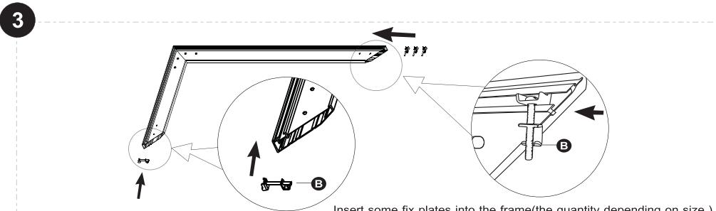
Insert some fix plates into the frame(the quantity depending on size )
